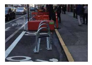
**F4. Bicycle parking:** Integrated bicycle parking is encouraged, especially on designated bike routes. Bicycle parking should be designed as an integrated element in the parklet design rather than as an 'add-on'.
